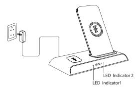
When the smartphone is on the dock, LED Indicator 1 will be white. When the Power Bank is on the dock, LED Indicator 2 will be white.
