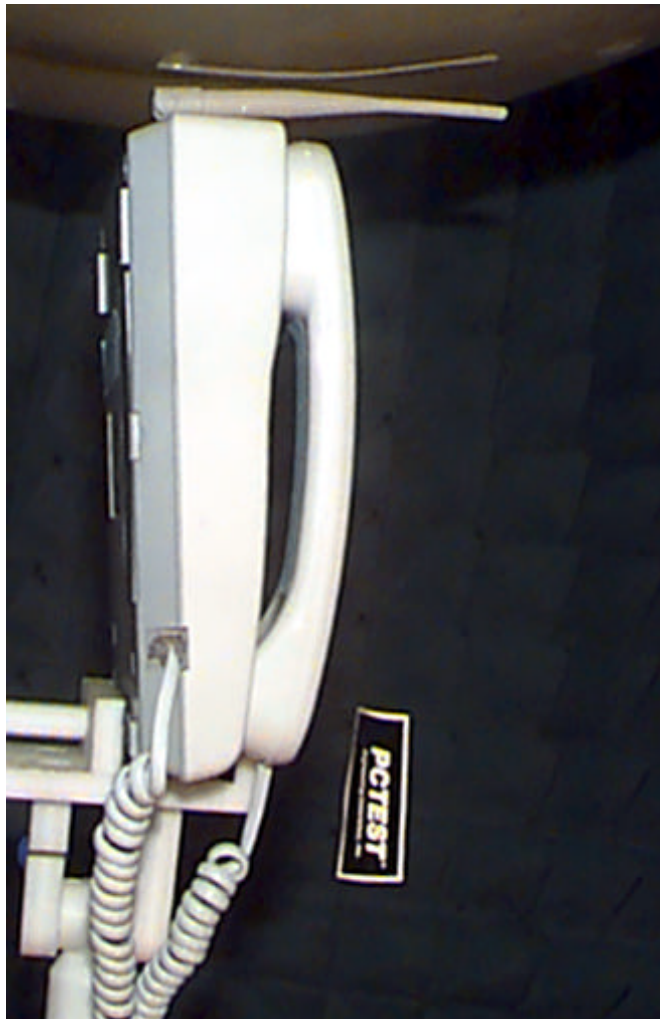
Figure 8. Test setup of EUT in normal operating position with the source of significant emissions (antenna) placed 2cm below the phantom.
