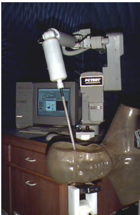
Figure 5. Photograph of the Probe and the Phantom
