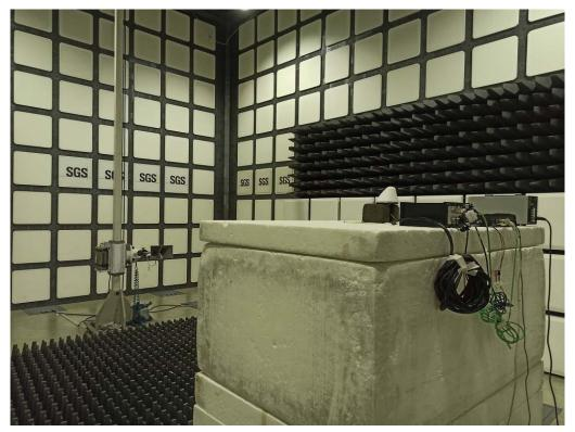
Radiated Emission Set up Photos (Front View)
