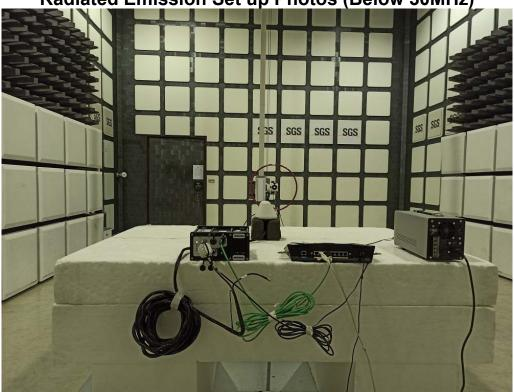
Radiated Emission Set up Photos (Below 1GHz)
