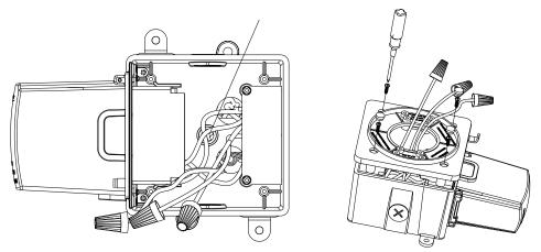
6. Fix the other fixing plate onto the back cover
