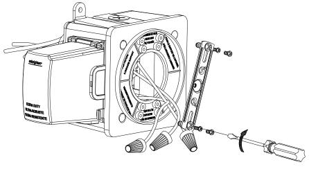
7. Connect the wires of junction box and light, then install the light on the fixing plate
