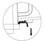
2. Connect the plug, need to open the cover, and take off the panel, then you can insert the plug into the outlet and close the cover.
