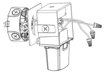
5. Fix the junction box and then install the back cover and tighten the screw.
