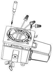
3. Install the fixing plate on to your existing junction box, if you don't have a junction box , can install the our junction box on the surface directly.
