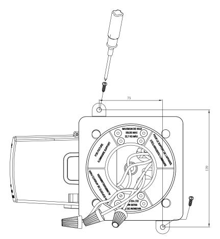
Use two screws to fix the junction box on surface via the two holes on the product
