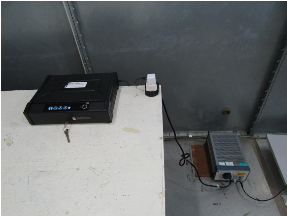
Measurement of Conducted Emission Test Set Up
