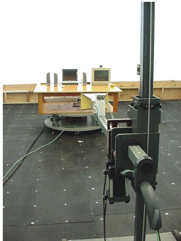
Photograph D.7-4 - Back of Radiated Emission Setup
