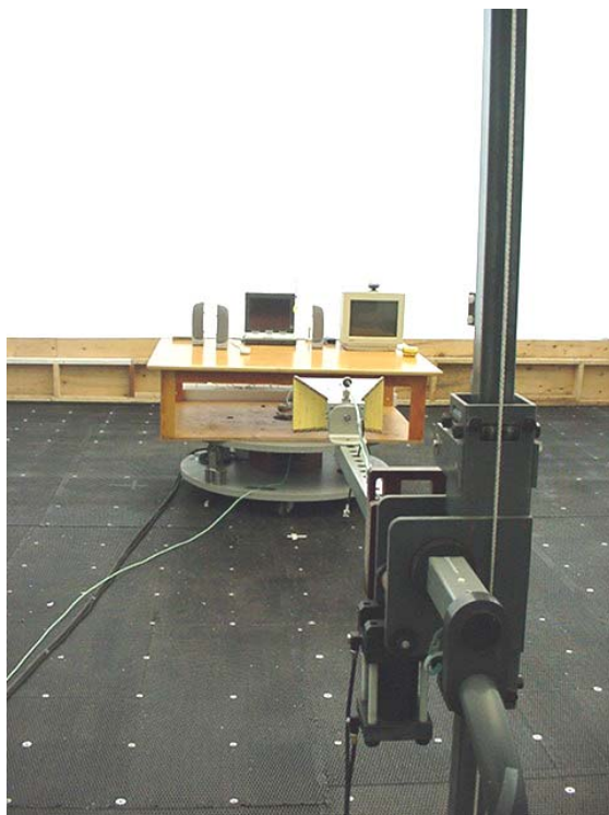
Photograph E.7-4 - Front of Radiated Emission Setup with vehicle-mount antenna and cradle
