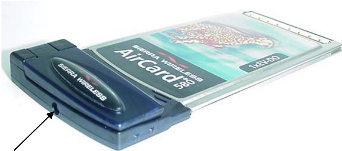
Photograph A.1-7 - AirCard 580 Dual-Band CDMA Modem
