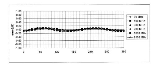
Axial Isotropy Error < ± 0.2 dB
