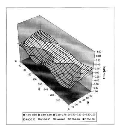
Spherical Isotropy Error < ± 0.4 dB
