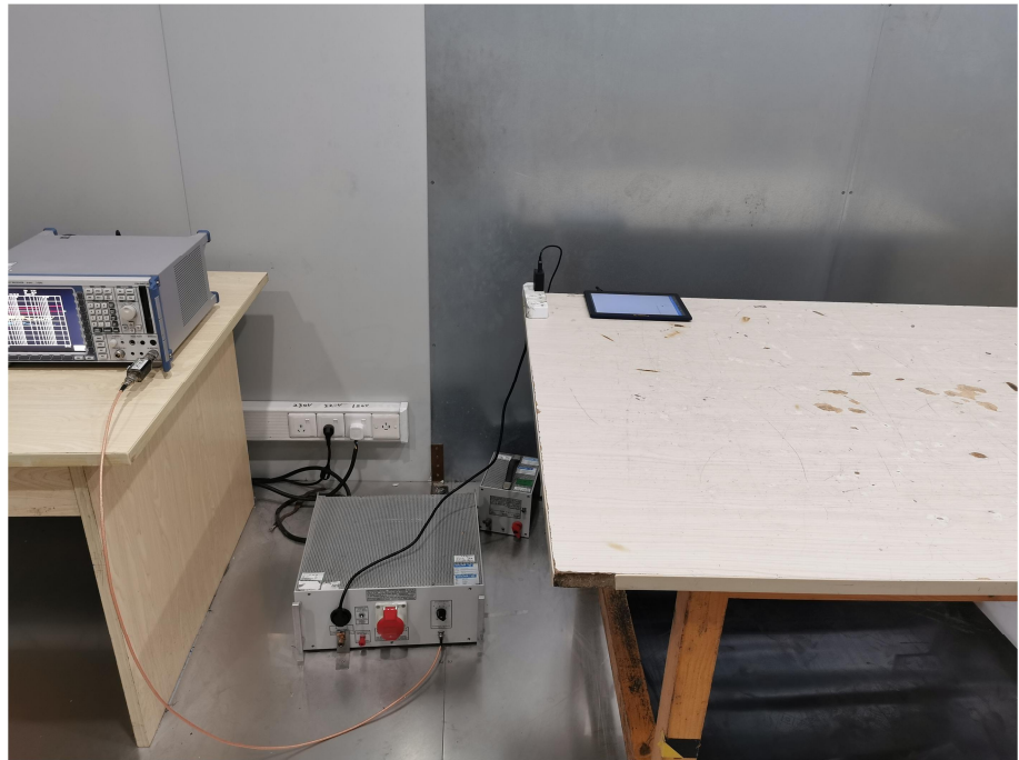
Conducted Emission Test Setup
