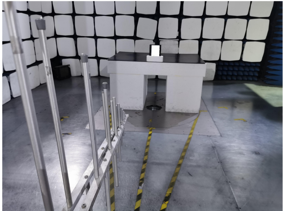
Radiation Emission Test Setup (30MHz to 1GHz)
