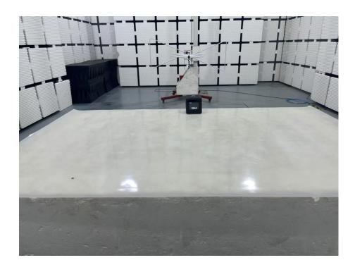
**Set-up for Radiated Spurious Emission, Above 1GHz**
