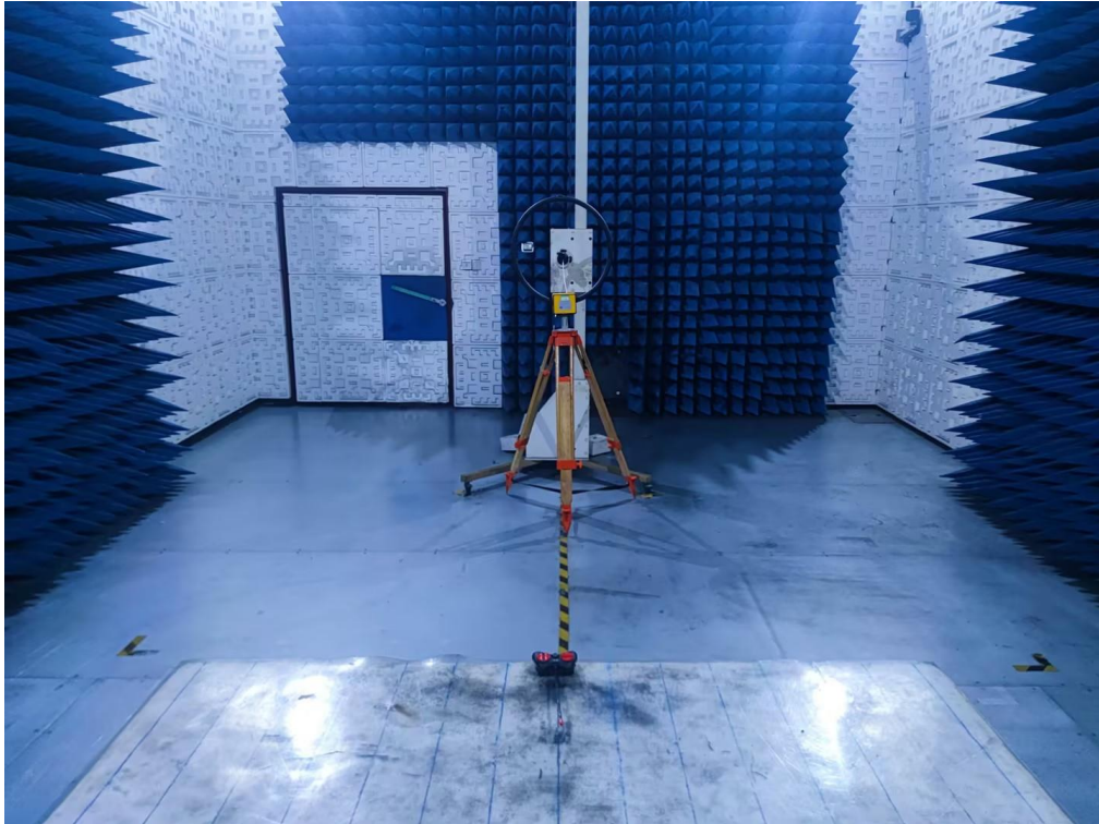
RADIATED EMISSION TEST SETUP BELOW 1GHz
