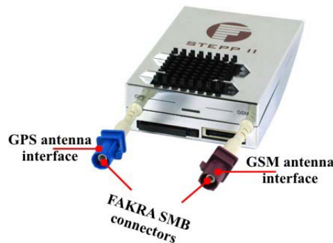
Figure 13: View of the GSM/GPS antenna cable.
