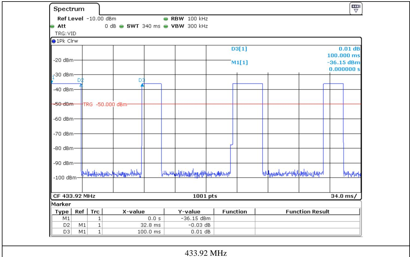
The average field strength may be found by measuring the peak pulse amplitude (in log equivalent units) and determining the duty cycle correction factor (in dB) associated with the pulse modulation as shown in Equation. (ANSI C63.10: 2013)
