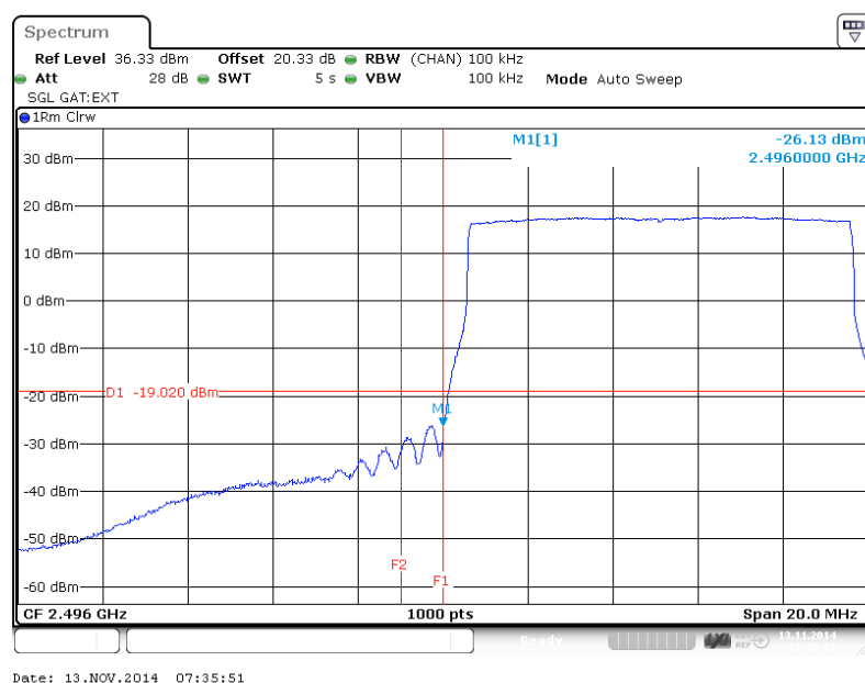
Figure 47 Spurious Emissions (Lower Band Edge) – QPSK (2501.1 MHz) (10MHz Channel BW)
