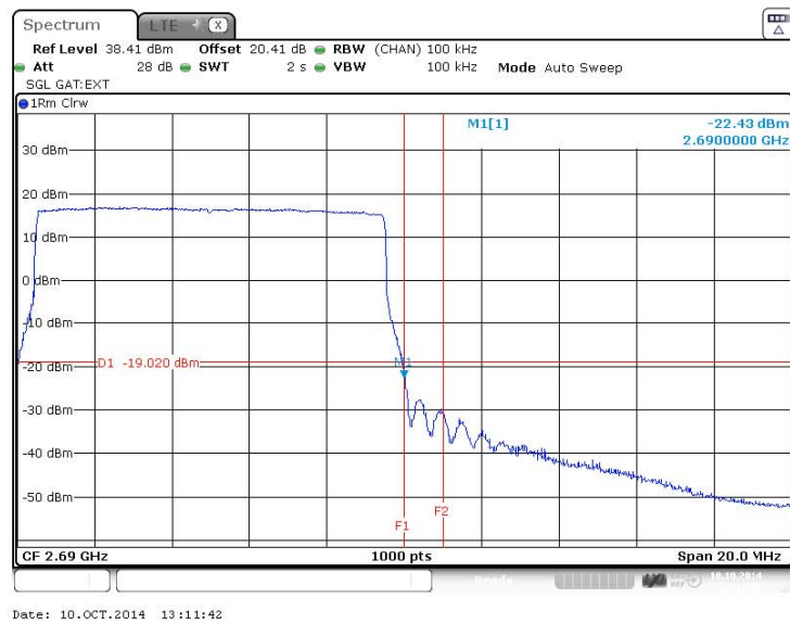
Figure 60 Spurious Emissions (Upper Band Edge) – QPSK (2685.0 MHz) (10MHz Channel BW)
