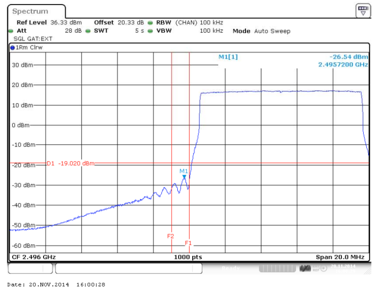
Figure 59 Spurious Emissions (Lower Band Edge) – QPSK (2501.1 MHz) (10MHz Channel BW)
