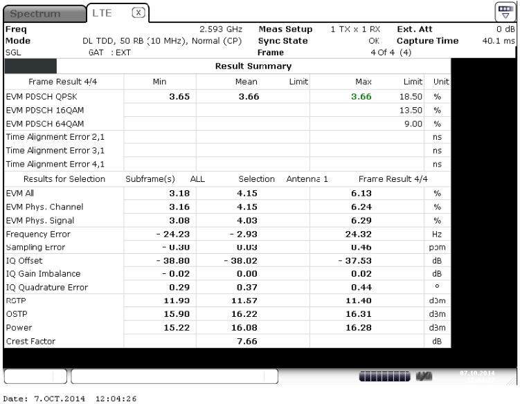
Figure 6 I/Q constellation table with I/Q error – QPSK (2593.0 MHz) (20MHz Channel BW)
