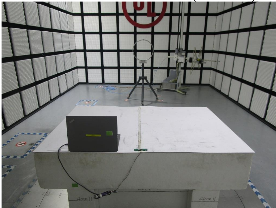
RADIATED RF MEASUREMENT SETUP (Below 30MHz)
