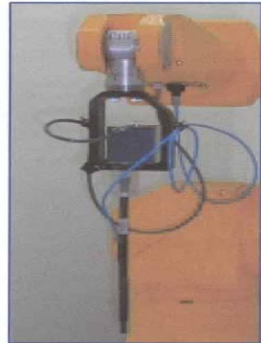
Figure4. ET3DV6 E-field probe
