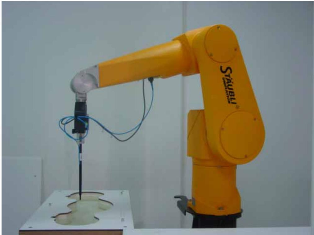
Picture 1 Specific Absorption Rate Test Layout
