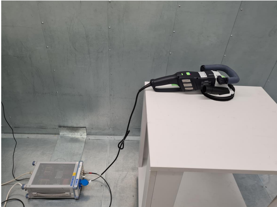
Figure 5: Conducted measurements test setup on AC mains
