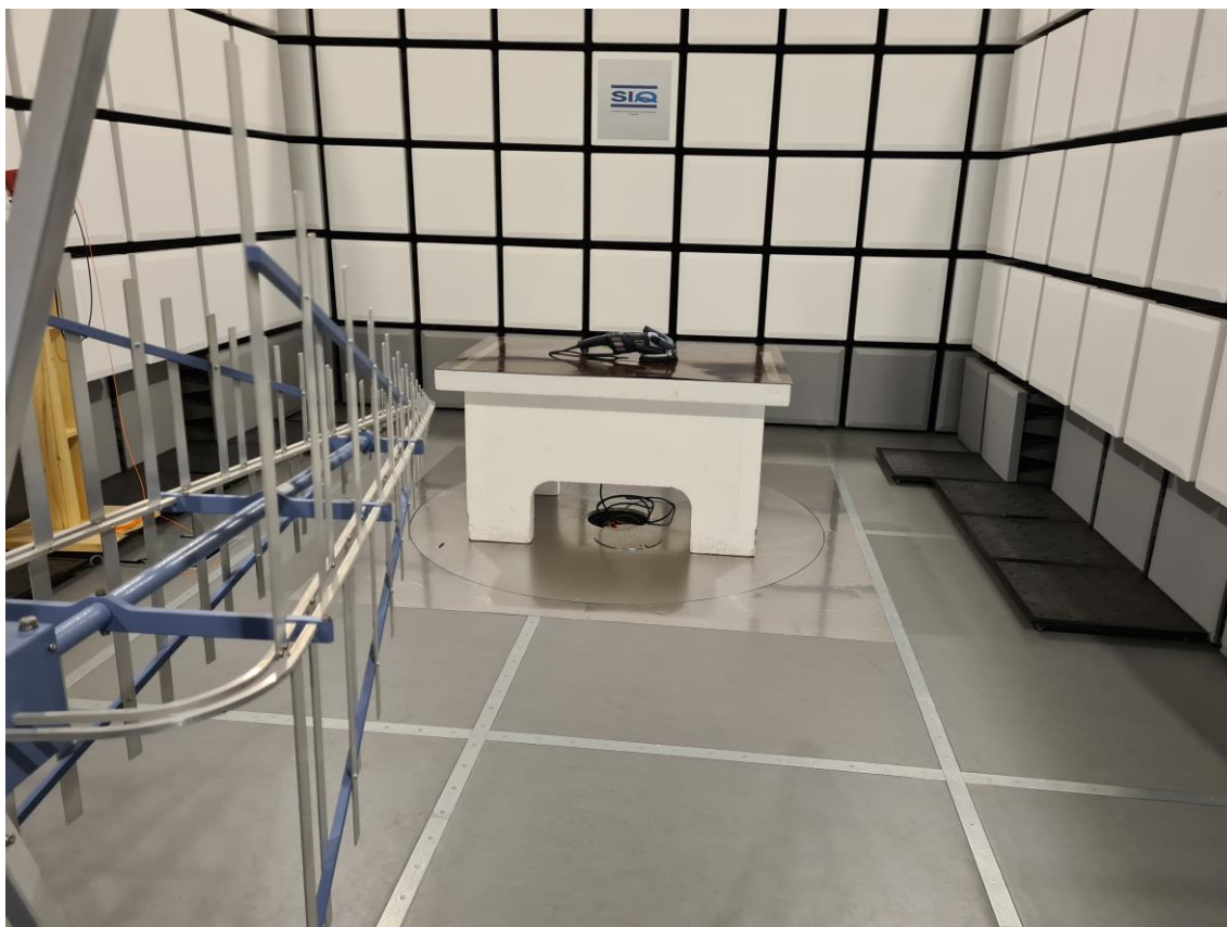
Figure 2: Spurious emission 30 MHz-1000 MHz
