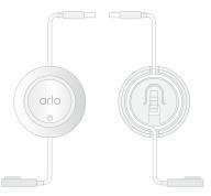
Snap the magnetic mount onto the screw and the stopper. The mount clicks into place.
