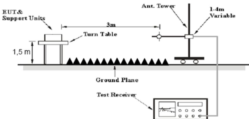
The radiated emission Below 1GHz tests were performed in the 3 meters chamber test site, above 1GHz tests were performed in the 3 meters chamber test site, using the setup accordance with the ANSI C63.10-2013. The specification used was the FCC 15.209, and FCC 15.247 limits and RSS-247 Clause 5.5, RSS-GEN Clause 8.10 limits.
