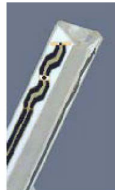
Figure 2.3 Probe Thick-Film Technique
