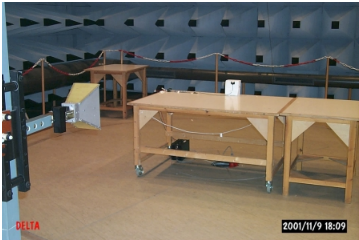
PHOTO A2.3 Test set-up for test 1-12.75 GHz
