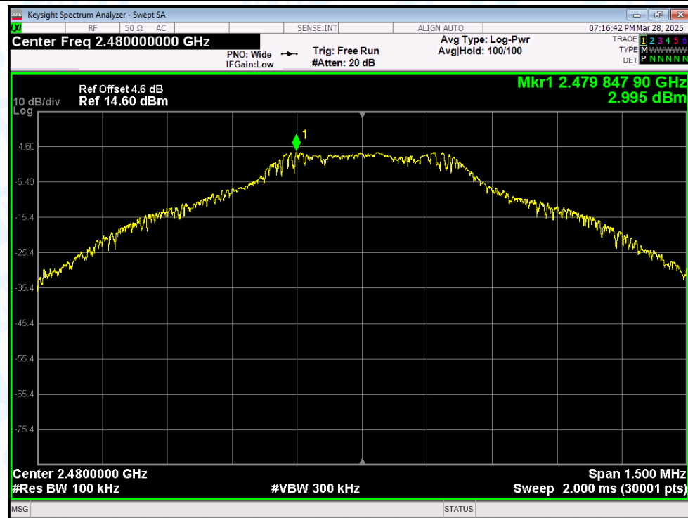
Tx. Spurious NVNT 1-DH1 2480MHz Ant1 Emission
