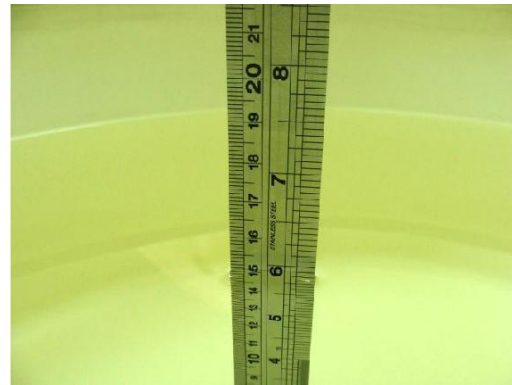
Fig 7.2 Photo of Liquid Height for Body SAR
