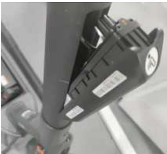
2. Install the cable of IoTbox into the groove of scooter's upright tube, beware to put the bottom part first, then comes the upper part.
