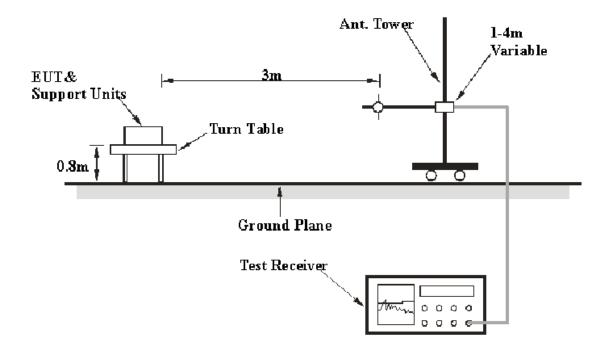
The radiated emission tests were performed in the 3-meter Chamber, using the setup accordance with the TIA/EIA 603-B. The specification used was the FCC 15.109 limits.
