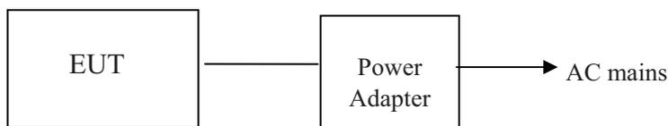
EUT was connected to control to a special test jig provided by manufacturer which has a USB connect to Notebook, and the Notebook will run a special test software provided by manufacturer to control EUT work in Continuous TX mode (>98% duty cycle), and select test channel, wireless mode and data rate.
