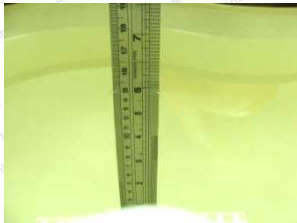
Photo of Liquid Height for Head SAR
