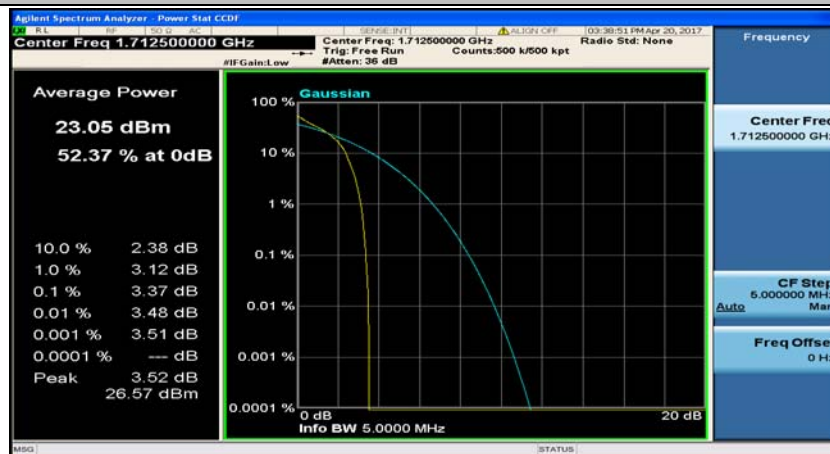
(Channel Bandwidth: 5 MHz)_LCH_QPSK_12RB#0
