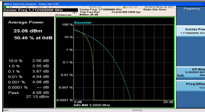
(Channel Bandwidth: 5 MHz)_LCH_QPSK_1RB#12
