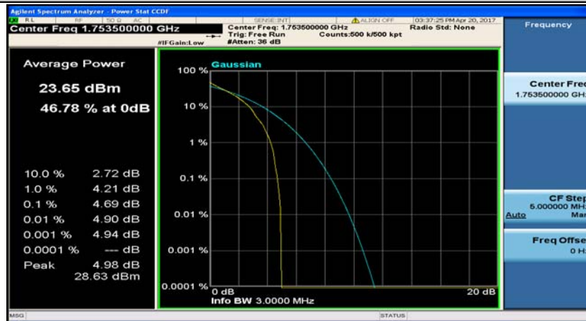
(Channel Bandwidth: 3 MHz)_HCH_QPSK_8RB#0
