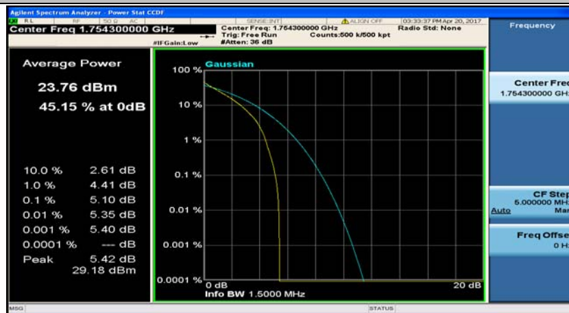
(Channel Bandwidth: 1.4 MHz)_HCH_QPSK_6RB#0
