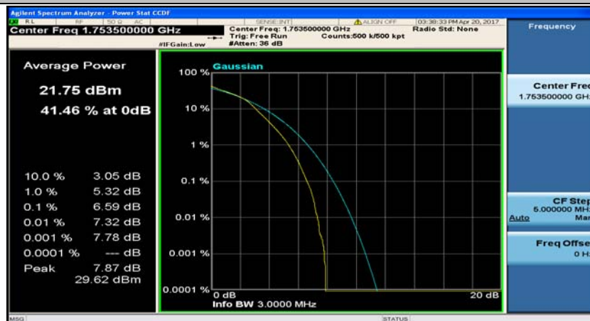
(Channel Bandwidth: 3 MHz)_HCH_16QAM_15RB#0
