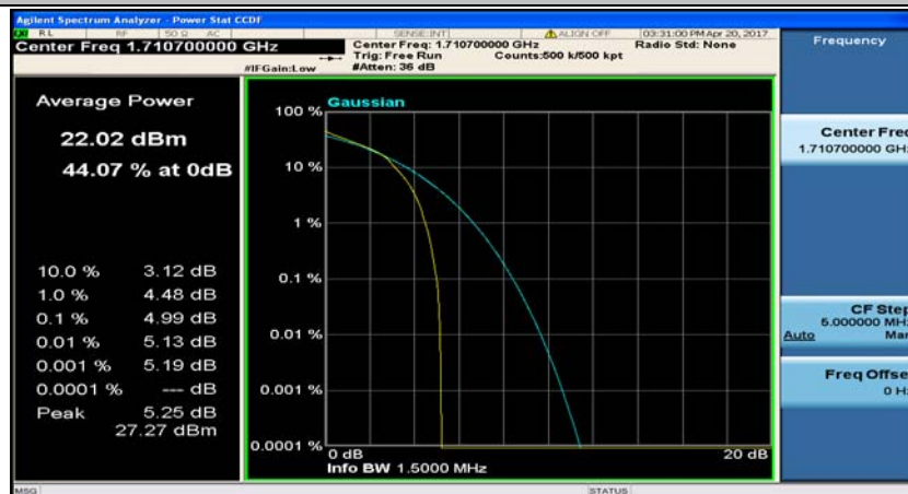
(Channel Bandwidth: 1.4 MHz)_LCH_16QAM_6RB#0
