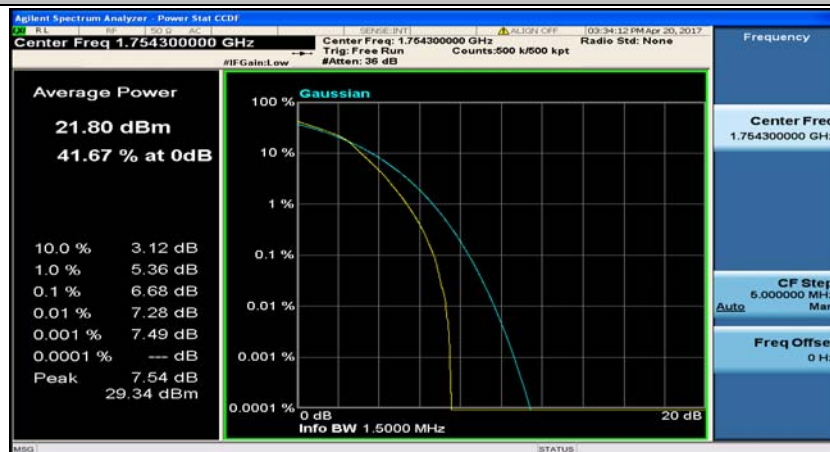
(Channel Bandwidth: 1.4 MHz)_HCH_16QAM_6RB#0
