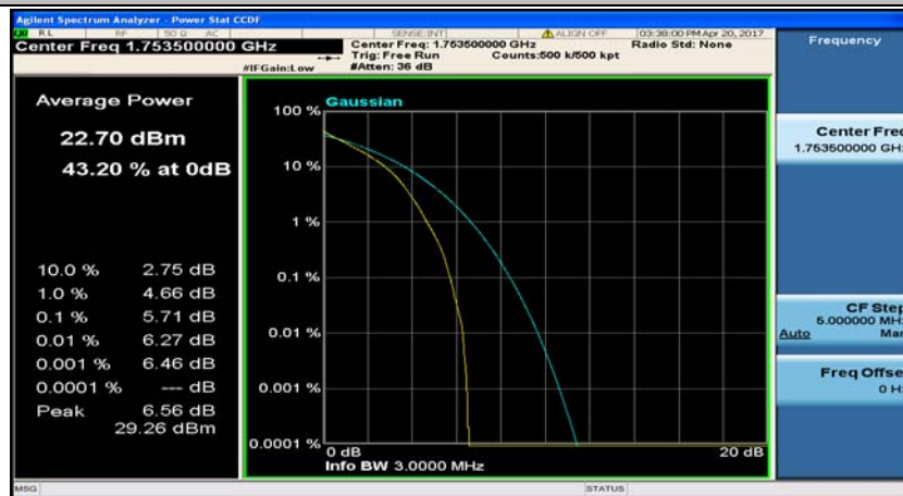
(Channel Bandwidth: 3 MHz)_HCH_QPSK_15RB#0
