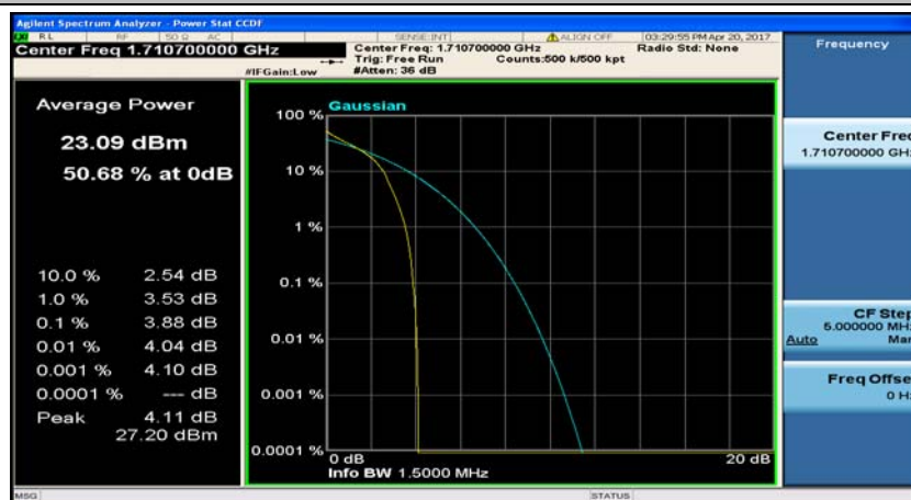
(Channel Bandwidth: 1.4 MHz)_LCH_QPSK_1RB#5
