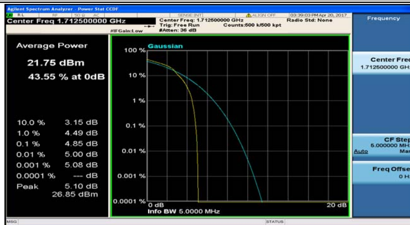
(Channel Bandwidth: 5 MHz)_LCH_16QAM_1RB#24
