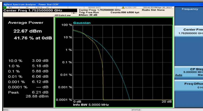
(Channel Bandwidth: 5 MHz)_HCH_16QAM_1RB#12
