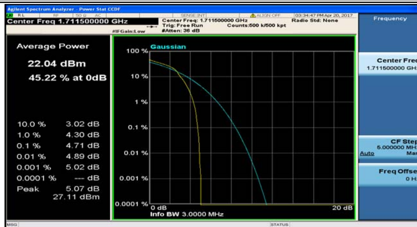
(Channel Bandwidth: 3 MHz)_LCH_16QAM_8RB#0
