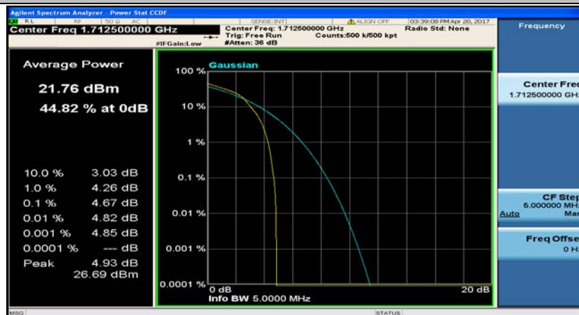
(Channel Bandwidth: 5 MHz)_LCH_16QAM_12RB#0
