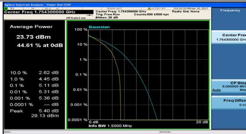
(Channel Bandwidth: 1.4 MHz)_HCH_QPSK_3RB#3
