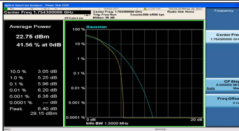
(Channel Bandwidth: 1.4 MHz)_HCH_16QAM_1RB#5
