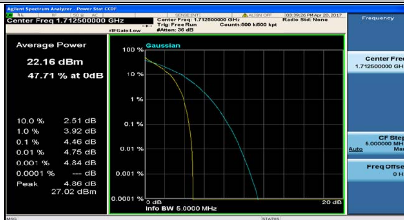
(Channel Bandwidth: 5 MHz)_LCH_QPSK_25RB#0
