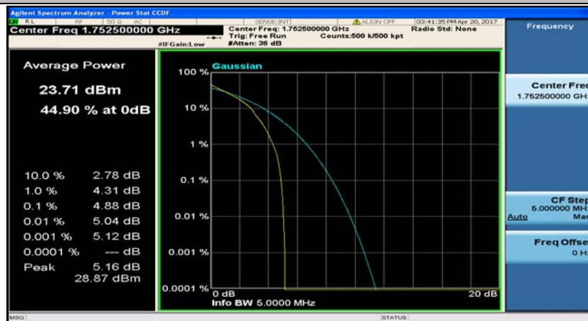
(Channel Bandwidth: 5 MHz)_HCH_QPSK_1RB#12
