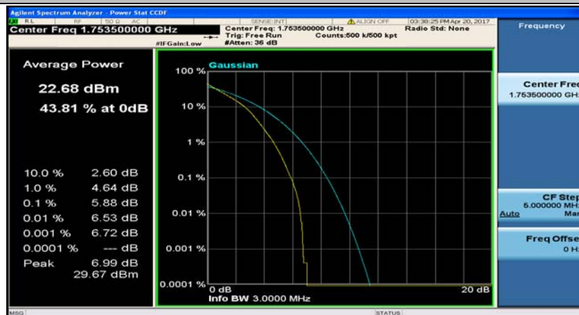
(Channel Bandwidth: 3 MHz)_HCH_QPSK_15RB#0
