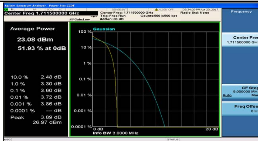
(Channel Bandwidth: 3 MHz)_LCH_QPSK_8RB#0
