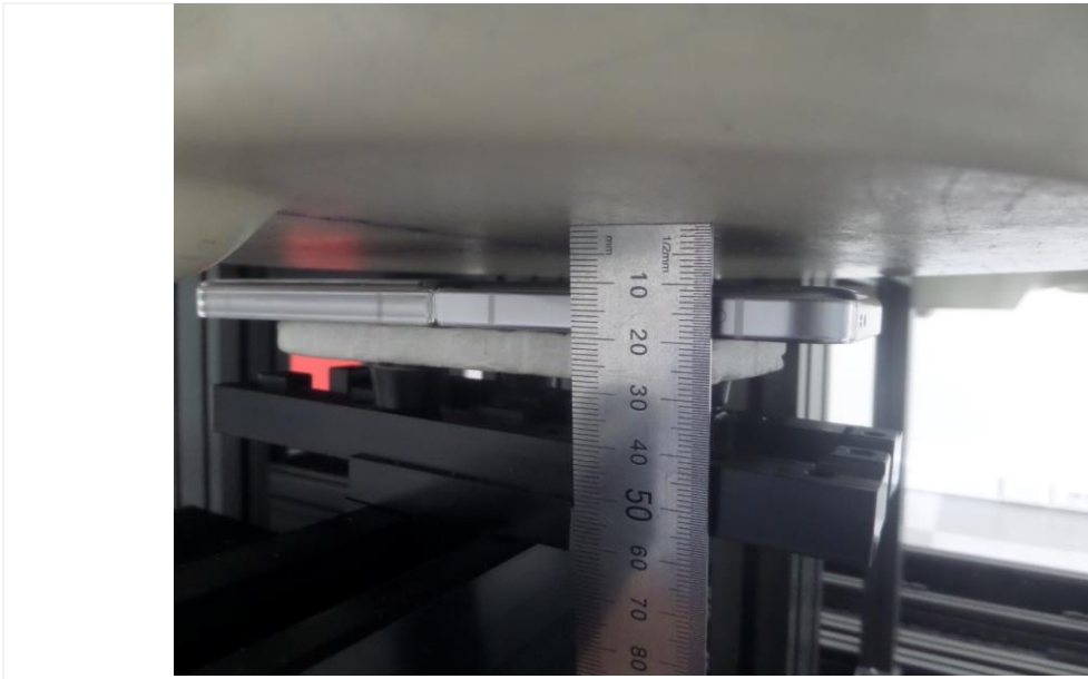
Distance of 10 mm from the EUT
