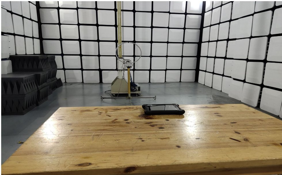
Photo of Radiation Emission Test
