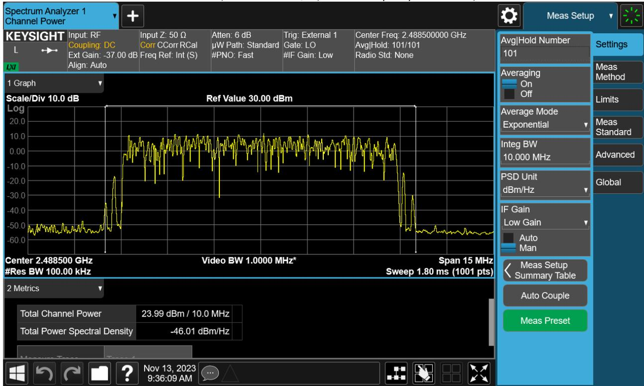
Test Model 3.1a, Modulation 256QAM, Channel Frequency 2490 MHz, TX1
