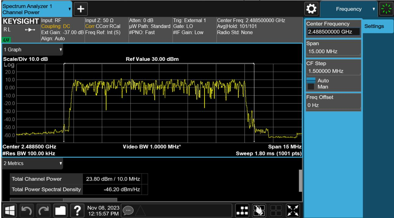
Test Model 3.1a, Modulation 256QAM, Channel Frequency 2490 MHz, TX3
