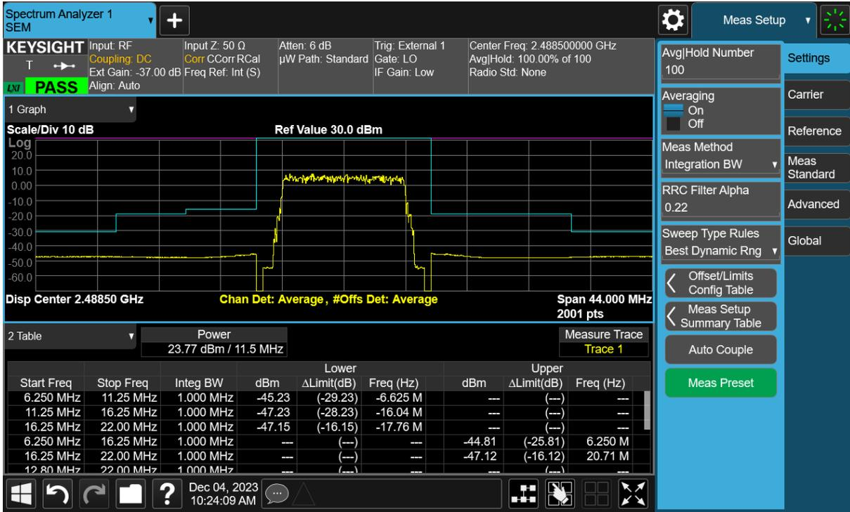
Test Model: 3.1a Modulation: 256QAM TX Port: 1 Channel Frequency MHz: 2490 Signal BW MHz: 10
