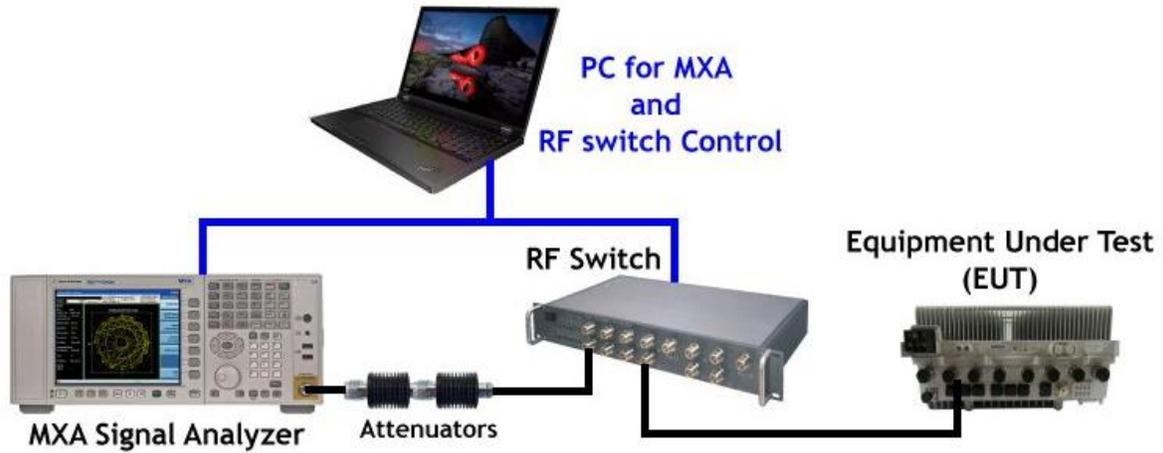
Test Setup for Frequency Stability
