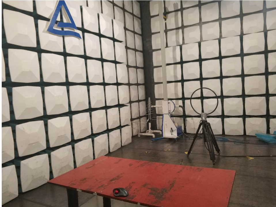
Photograph 1: Set-up for Radiated Spurious Emission, 9kHz - 30MHz
