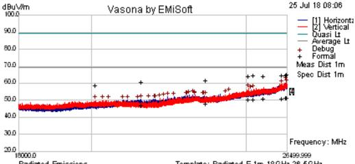
Radiated Emissions Template: Radiated E 1m 18GHz-26.5GHz Filename: c:\program files\emisoft - vasona\results\femtocell\_2018-0148\_0147\RE18-26.5GHz \
