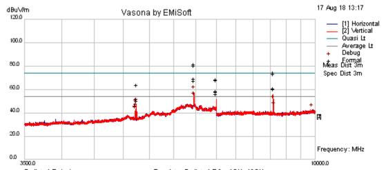
Radiated Emissions Template: Radiated E 3m 1GHz-18GHz
