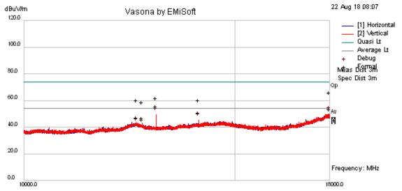
Radiated Emissions Template: Radiated E3m 1GHz-18GHz
