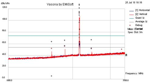
Radiated Emissions Template: Radiated E 3m 1GHz-18GHz
