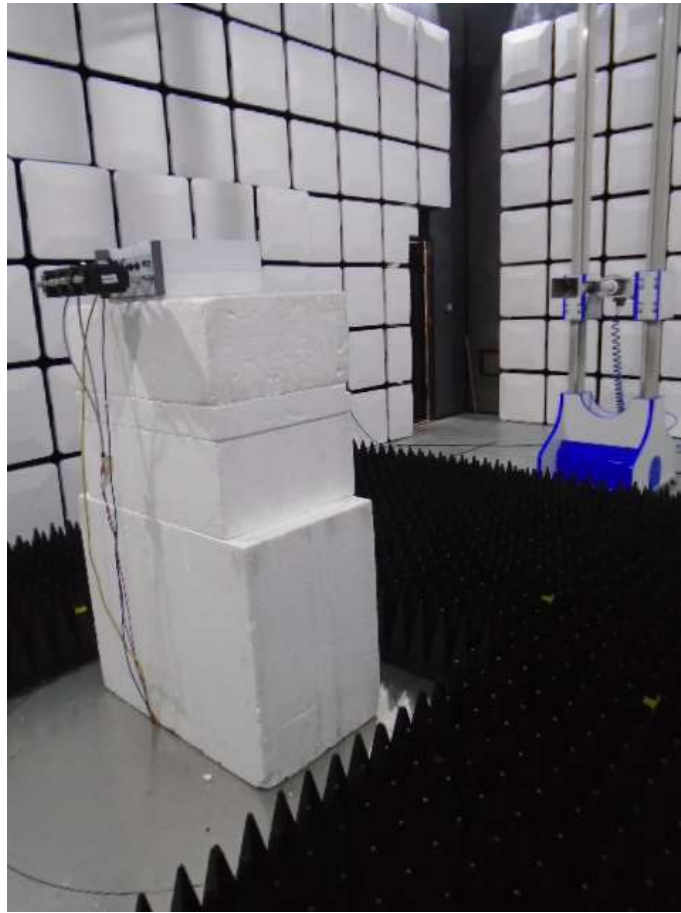
Radiated 1GHz – 8GHz Testing
