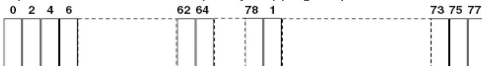
Each frequency used equally on the average by each transmitter. The system receivers have input bandwidths that match the hopping channel bandwidths of their corresponding transmitters and shift frequencies in synchronization with the transmitted signals.
