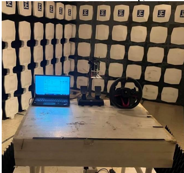
Measurement of Radiated Emission Test Set Up(Above 1000MHz)
