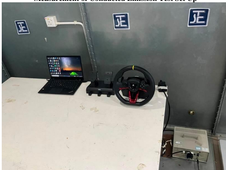
Measurement of Conducted Emission Test Set Up
