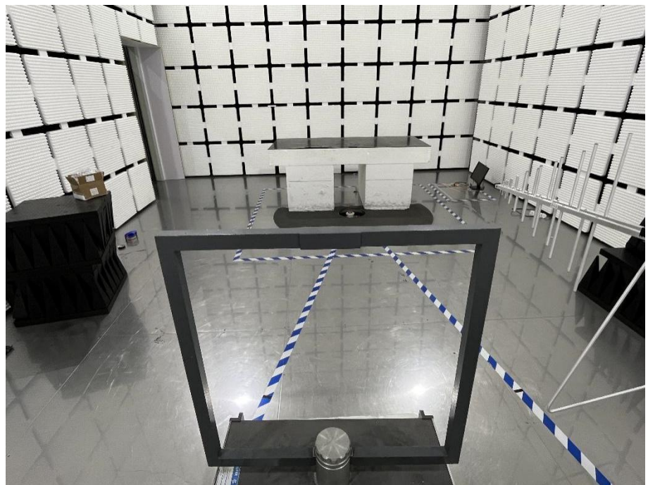
Radiation Emission Test Setup (Below 30MHz)
