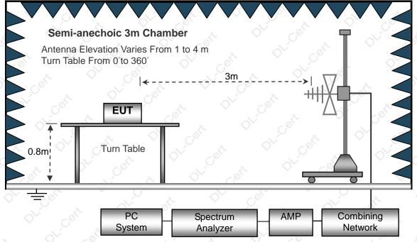
(C) Radiated Emission Test-Up Frequency Above 1GHz
