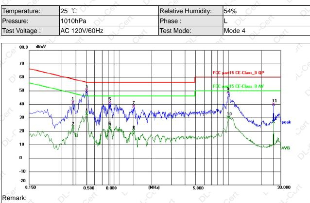
Margin = Limit – Level, Correct Factor = Cable lose + LISN insertion loss, Level= Reading + Correct factor
