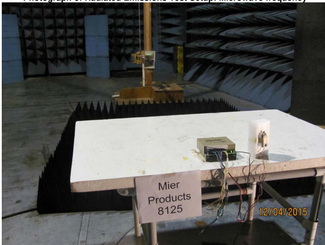
Photograph of Radiated Emissions Test Setup: Microwave frequency
