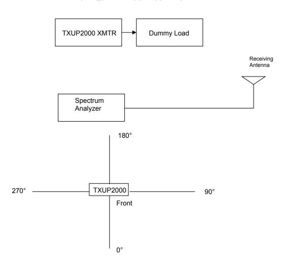
As indicated in the spreadsheet data, the worst case calculation was 72.6 dB at the tenth harmonic. The measurement tables for the all views of the transmitter at each frequency are shown below. The results indicate that all radiated harmonics meet the FCC requirement of 60 dB as outlined in FCC rule 2.1053 and 2.1057.
