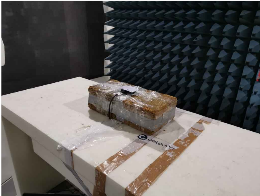
Photograph 1: EUT test setup 2 in the semi anechoic chamber, close up view_EUT elevation 0°, EUT in TXRX mode
