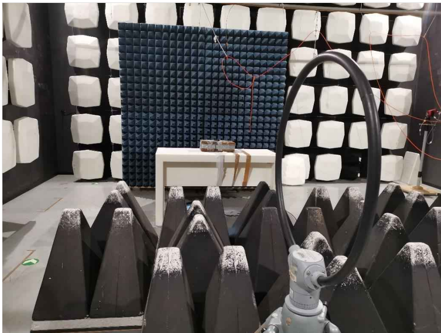
Photograph 2: EUT test setup 1 in the semi anechoic chamber, overview_EUT elevation 0°, EUT in TX mode
