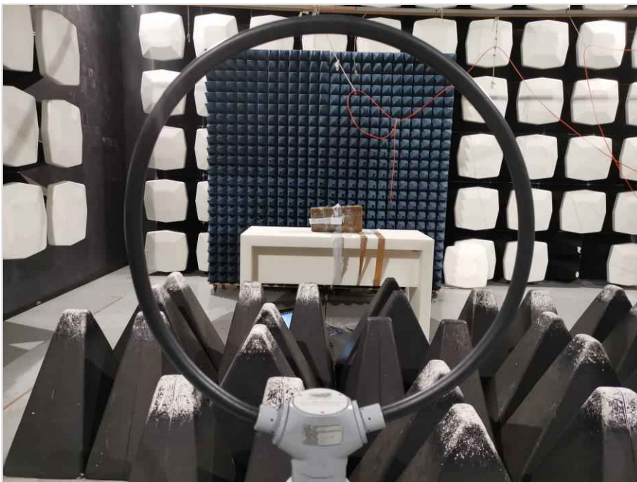
Photograph 4: EUT test setup 2 in the semi anechoic chamber, close up view_EUT elevation 90°, EUT in TXRX mode
