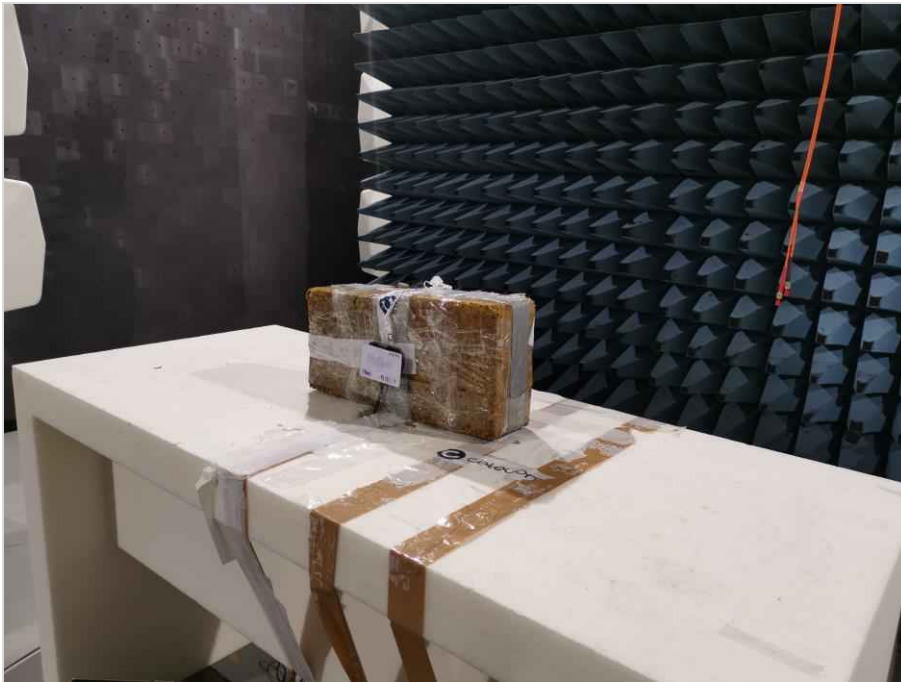
Photograph 3: EUT test setup 2 in the semi anechoic chamber, close up view_EUT elevation 90°, EUT in TXRX mode
