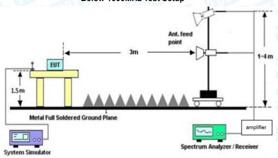
**Above 1GHz Test Setup**
