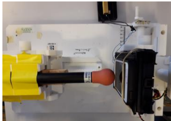
Top View of E/B Wavecontrol probe and EUT.
