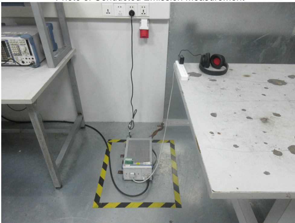
FCC ID: WSG-H7 Photo of Conducted Emission Measurement
