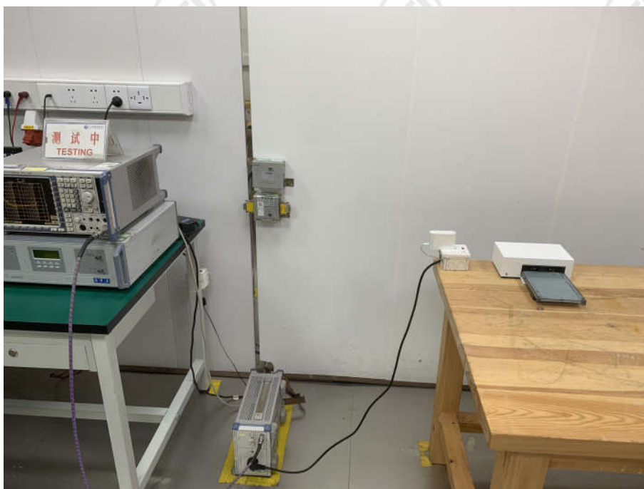
AC Power Line Conducted Emission
