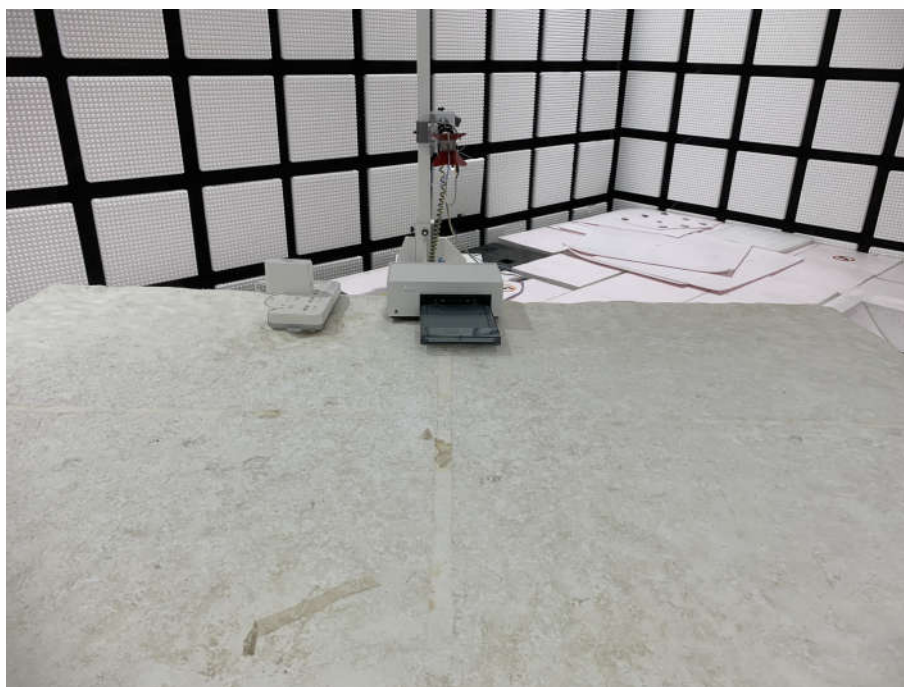
Radiated spurious emission Test Setup-2(Above 1GHz)
