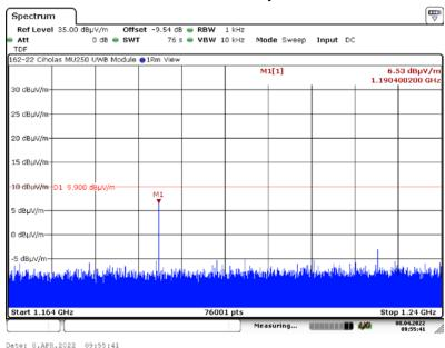
6.5.4.4 Vertical Measurement Polarity 1164 to 1240 MHz - 64M PRF
