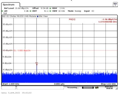
6.5.5.2 Vertical Measurement Polarity 1559 to 1610 MHz - 16M PRF
