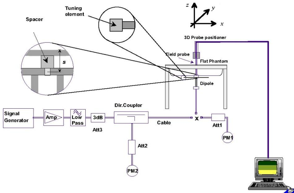
The output power on dipole port must be calibrated to before dipole is connected.
