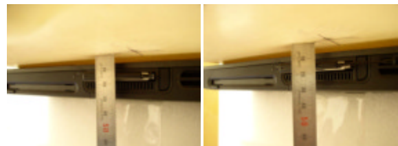
Fig. 20. Body SAR Test Setup with Holster
