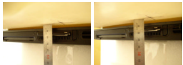
Fig. 21. Body SAR Test Setup with Holster
