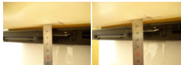
Fig. 18. Body SAR Test Setup with Holster
