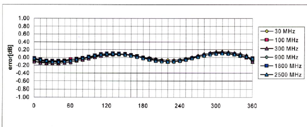
Axial Isotropy Error <  $\pm 0.2$  dB
