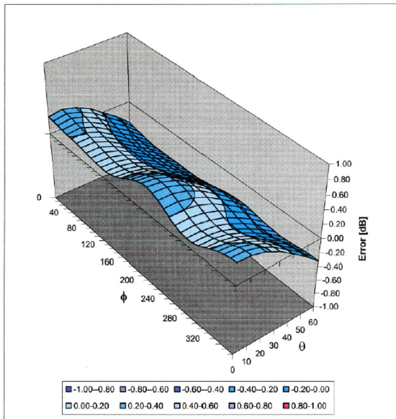
Spherical Isotropy Error < ± 0.4 dB
