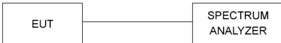
Figure 1 - Bandwidth Measurements Test Setup
