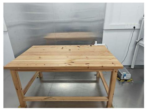
**Radiated Emission Test View Below 1GHz**
